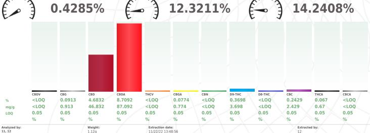
Analysis Method: N/A Analytical Batch: CE001629POT Instrument Used: HPLC 2040 EID 184
