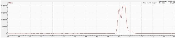
The prominent peak at 5.2 min is characterized by m/z 317 and the full scan spectrum is characterized by ions at m/z 2898 271, and 201.
