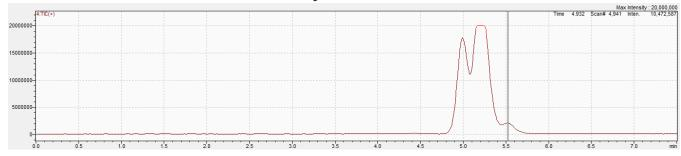
The prominent peak at 5.5 min is characterized by m/z 317 and the full scan spectrum is characterized by ions at m/z 289, 270, and 200.
