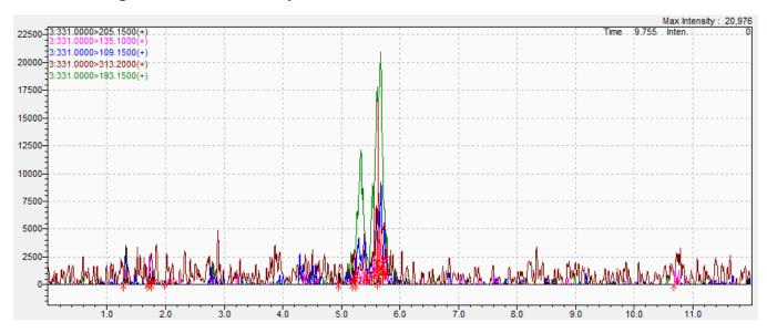
Nothing was identified in this ion chromatogram. The ions are of low intensity and probably do not represent substantial products.
