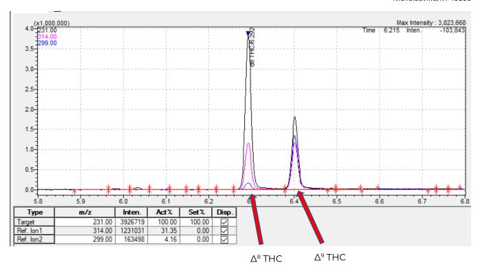
The following is a SIM analysis of Sample 2132 showing ions and retention times for  $\Delta^8$ -THC and  $\Delta^9$ -THC. The table below the ion chromatogram reports the relative abundances of the most abundant ion for  $\Delta^8$ -THC at m/z 231, the molecular ion at m/z 314, and a major fragment ion at m/z 299.
