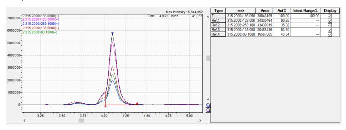
The presence of  $\Delta^8$ -THC was confirmed by the ions and ion area ratios of the peak at 4.10 minutes in sample #2132. The peak just to the left of the peak for  $\Delta^8$ -THC has ions characteristic of  $\Delta^9$ -THC but we do not believe that identification criteria were met for this identification.
