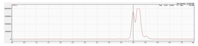
The prominent peak at 5.0 min is characterized by m/z 317 and the full scan spectrum is characterized by ions at m/z 289, 270, and 201.
