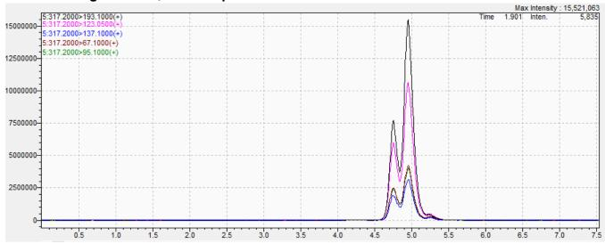
These peaks have masses and fragmentation patterns similar to those of CBG but the retention times are incorrect for CBG. The apparent molecular mass of the three substances eluting between 4.5 and 5.3 minutes is 316. This mass is identical to that of various isomers of hexahydrocannabinol.
