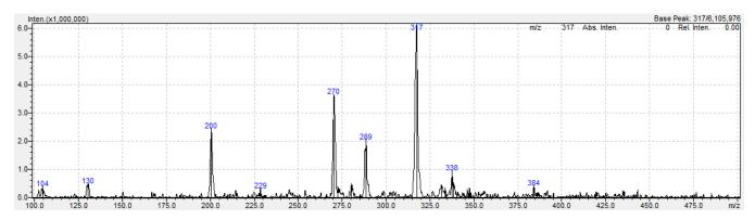
The product ion scan for m/z 317 at 5.5 min is characterized by fragment ions at m/z 194 and 124.
